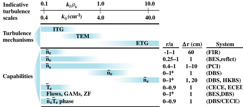
**Figure 3.** Multifield and multiscale fluctuation diagnostics on DIII-D. The figure compares the wavenumber ranges of representative instabilities with the diagnostic wavenumber range. Diagnostic system, measurement, approximate spatial coverage and spatial resolutions are also indicated.
