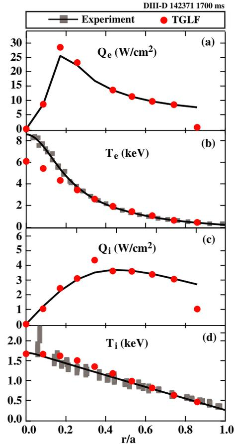
**Figure 11.** Flux matched transport solutions using the TGYRO/TGLF model for high  $T_e/T_i$  case. (a), (c) are electron and ion thermal fluxes, experiment is a solid line, model is filled circles, (b), (d) are comparisons of measured (squares) and predicted (circles) electron and ion temperature profiles.
