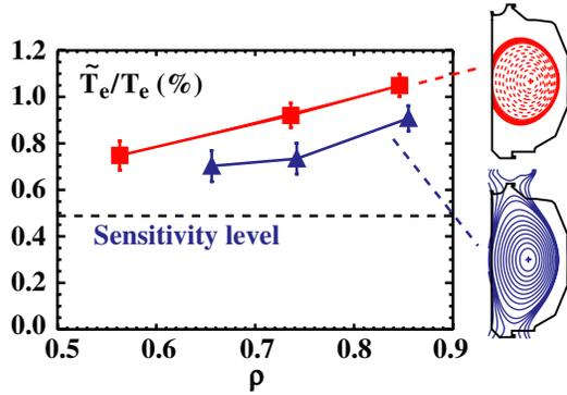
**Figure 2.** Variation in  $\tilde{T}_e/T_e$  measured by CECE with radial position and plasma elongation.
