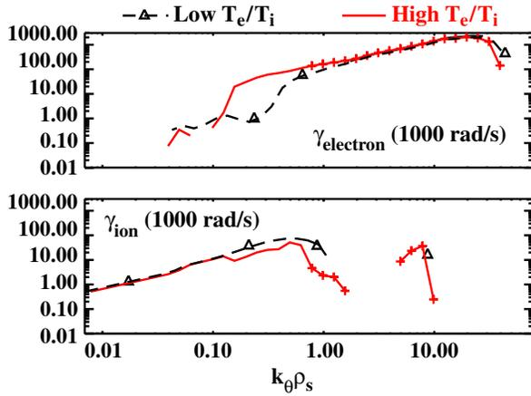
**Figure 6.** Linear growth rates for radial location  $\rho = 0.6$  from the TGLF code for ion and electron modes versus wavenumber for low and high  $T_e/T_i$  cases.
