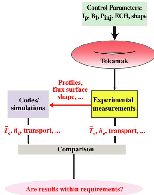
**Figure 1.** Validation procedure highlighting experimental input to the simulations and comparison of measurements (e.g.  $\tilde{T}_e/T_e, \tilde{n}_e/n_e$ , transport, etc). After the last step an iteration cycle can be commenced by varying one or more of the simulation input parameters (e.g. temperature and density scale lengths, temperatures, flow velocity, etc, re-running the simulation and comparing the new results with experiment).
