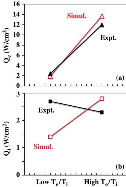
**Figure 8.** Simulation and experiment (a) electron and (b) ion thermal fluxes at  $\rho = 0.6$  in physical units for low and high  $T_e/T_i$  cases.
