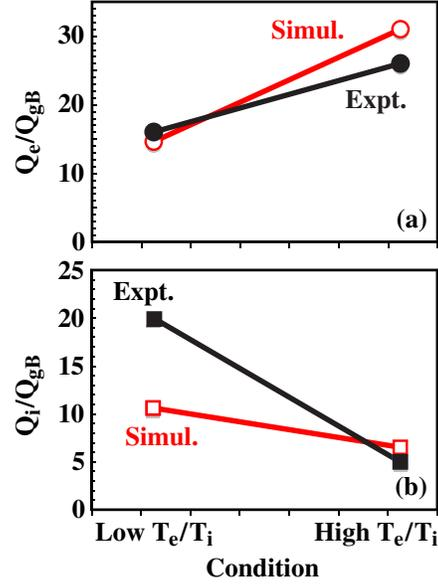
**Figure 7.** Simulation and experiment (a) electron and (b) ion thermal fluxes at  $\rho = 0.6$  normalized to gyro-Bohm flux,  $Q_{gB} = n_e c_s T_e$  for low and high  $T_e/T_i$  cases.
