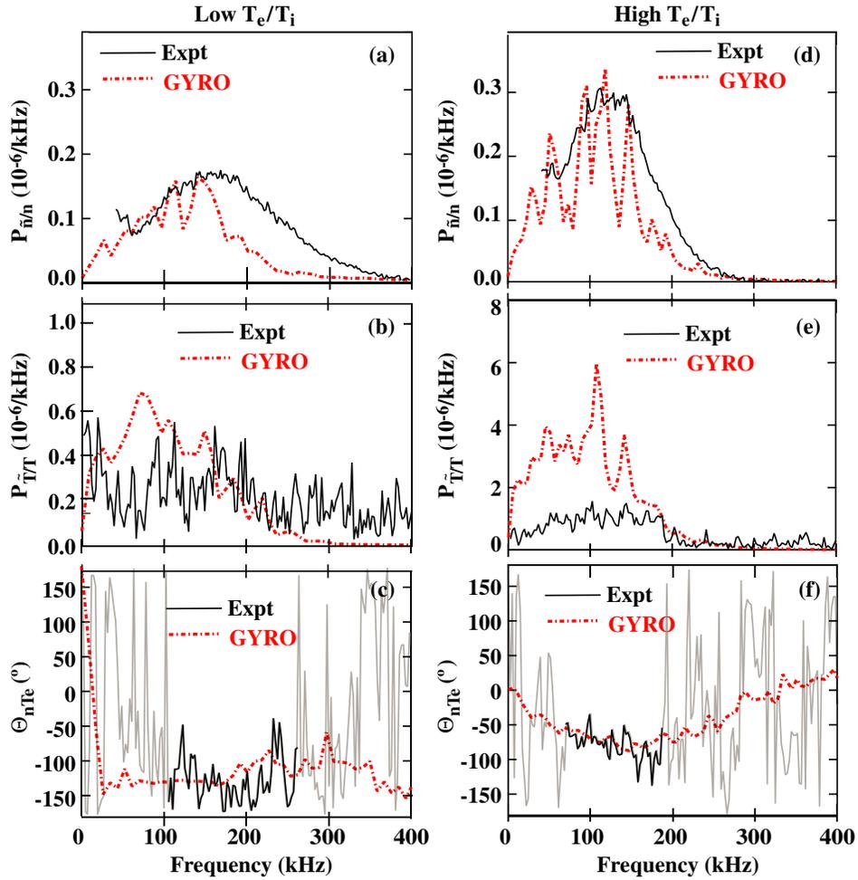
**Figure 9.** Measured and GYRO simulated power spectra at radial location  $\rho = 0.6$  for electron density fluctuation levels  $(\tilde{n}/n)^2$  (a), (d), electron temperature fluctuation levels  $(\tilde{T}_e/T_e)^2$  (b), (e), and electron density–temperature fluctuation cross phase  $\Theta_{nT}$  (c), (f). Left and right hand columns are low and high  $T_e/T_i$  cases, respectively.
