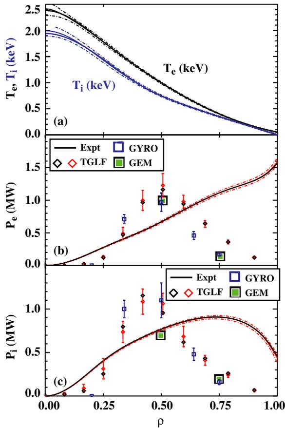
**Figure 12.** (a) Experimental  $T_e$ ,  $T_i$ , (b) experimental and predicted electron energy flow through the local surface area ( $P_e$ ), (c) experimental and predicted ion energy flow through the local surface area ( $P_i$ ).
