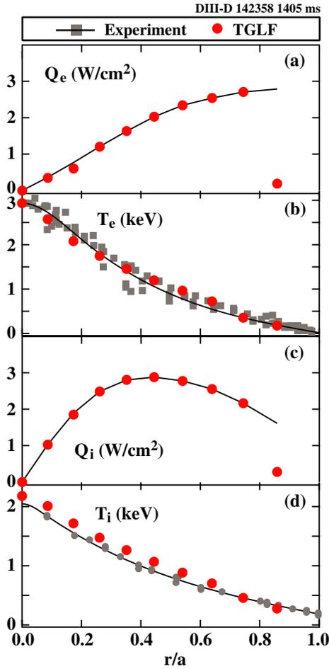
**Figure 10.** TGYRO/TGLF model transport matched (also termed flux matched) solutions for low  $T_e/T_i$  case. (a), (c) are electron and ion thermal fluxes, experiment is a solid line, model is filled circles, (b), (d) are comparisons of measured (squares) and predicted (circles) electron and ion temperature profiles.
