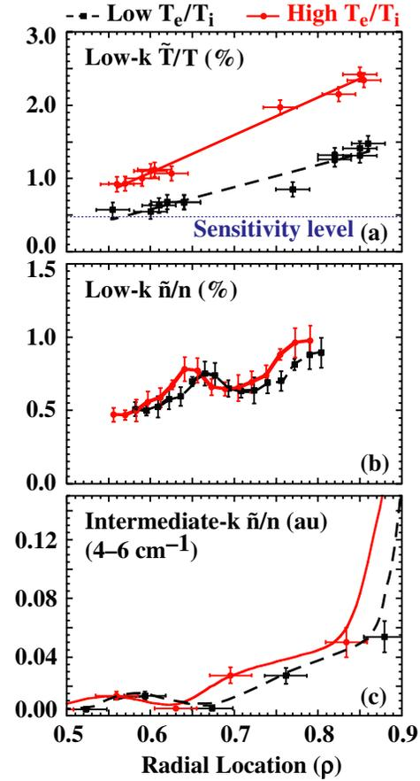
**Figure 5.** Experimental measurements: radial profiles of (a) low- $k$   $\tilde{T}_e$  (CECE), (b) low- $k$   $\tilde{n}$  (BES) and (c) intermediate- $k$   $\tilde{n}$  (DBS) for low and high  $T_e/T_i$  cases. Solid lines are guides for the eye.
